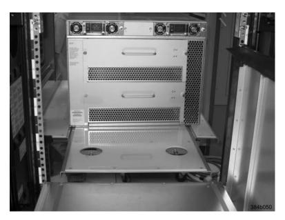
Figure 12. Load plate extended inside the cabinet to the exhaust kit shelf
